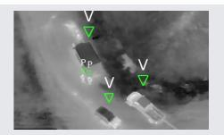
The system can recognize targets up to 400m away and detect them using infrared thermal imaging at a range of 1,600m for precise strikes. Attack Accuracy is CEP<1m.
