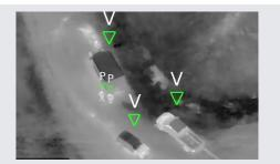
The system can recognize targets up to 400m away and detect them using infrared thermal imaging at a range of 1,600m for precise strikes. Attack Accuracy is CEP<1m.
