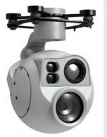
Gain the advantage with exceptional detection capabilities—identify personnel up to 37.5 km, small vehicles at 115 km, and large vehicles at 245 km. For precise identification, count on recognition ranges of up to 9.3 km for personnel and over 60 km for larger targets. Featuring a 4.09-million-pixel sensor with powerful 30× optical and 4× digital zoom, this system delivers crystal-clear imagery even at extreme distances.
